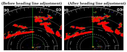
The bow of the ship is lined up with the tip of the peninsula (left), but the green heading line is not. Adjusting the heading line will allow you to align the direction of the heading line with the direction of the bow (right).
